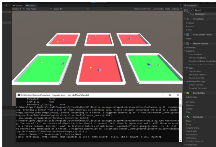
Fig. 4. The process of parallel training of an agent on 6 environments
